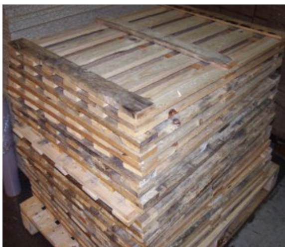
Example of wooden board to be used when double stacking.
