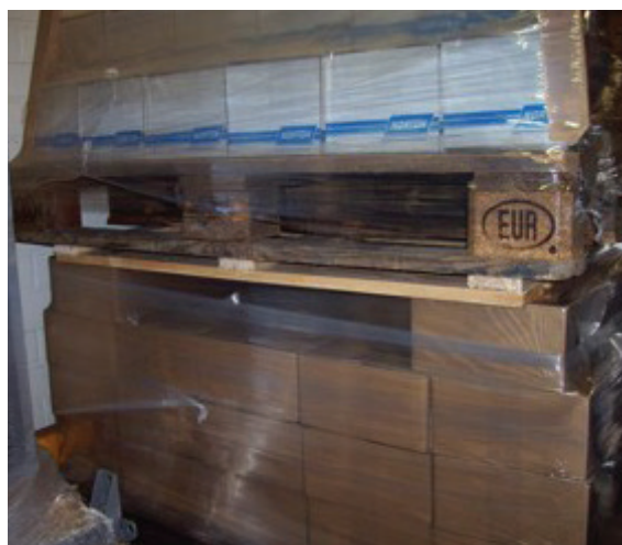
Use wooden board to separate the pallets.
