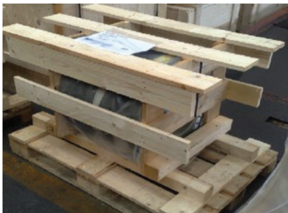
Example of good vertical pallet packing.
